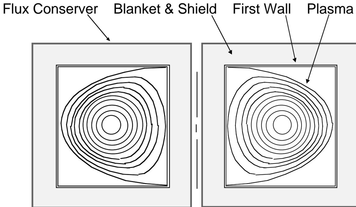
Figure 2. Hypothetical fusion reactor based on the use of self-generated magnetic fields. The ports for vacuum pumping, wave injection, and diagnostics are not shown.
