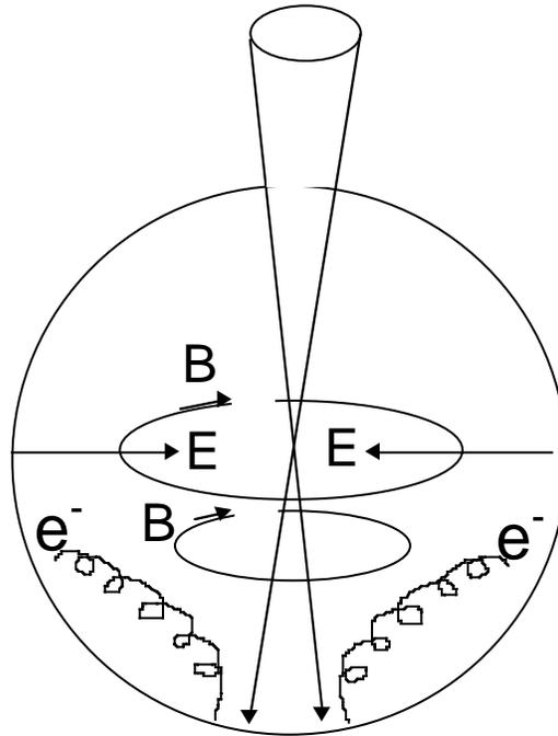
Figure 1. Generation of a magnetic field by a laser beam injected into a spherical metal shell. (After Hasegawa et al., 1988)
